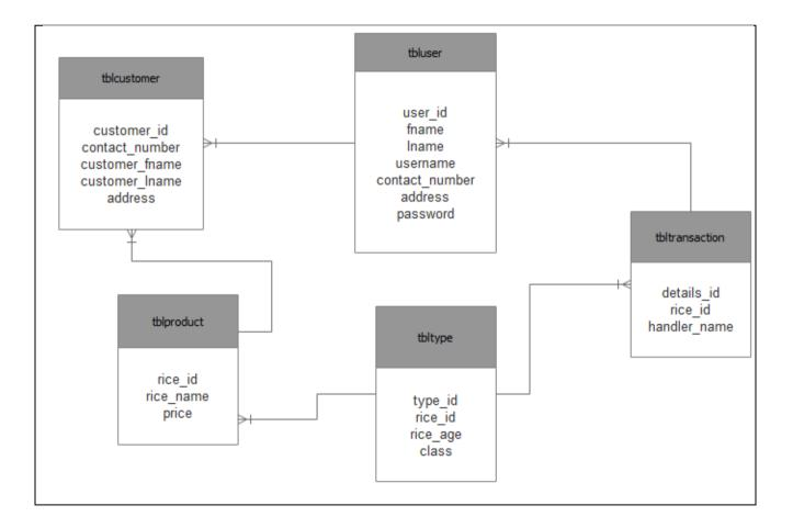
Figure 1: Proposed Rice Delivery and Inventory System Entity Relationship Diagram
